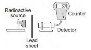
One lead sheet, 2 mm thick, was placed between the source and the detector and a count rate was taken. Extra lead sheets were added. For each extra lead sheet, a new count rate was taken and recorded in the table.
